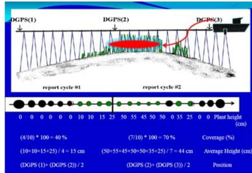
As transects are driven over during pesticide applications, the echosounder system automatically records bottom depth and plant canopy height and density. The data collected is time-stamped, geo-referenced and digitally stored. This system allows for the data to be collected during treatment, so real time plant data is available to support post treatment efficacy evaluations.
